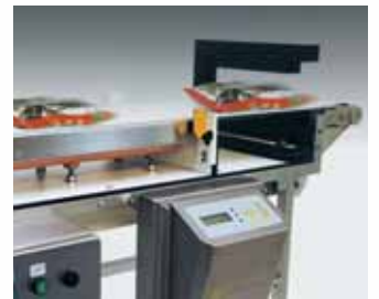
Detection of foreign objects even through aluminum packaging
